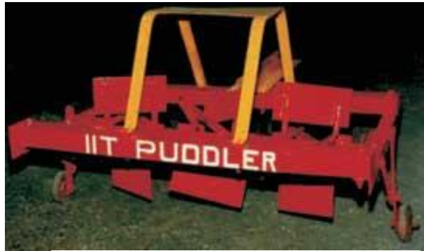
Improved device for wet soil preparation
